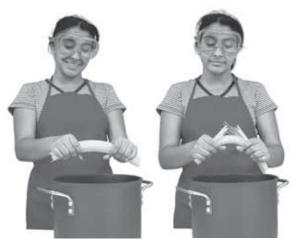
How can the same material bend in one situation but break in another? The answer is that the stress on the material is different in each case. *Stress* is the amount of force per unit area that is placed on an object.  $\blacksquare$
